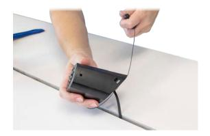
Alternate pulling the removal tool handles with each hand, in a sawing motion, until the pedestal is detached.
