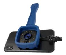
To remove the sensor from the device, place VP-1477 removal tool over the sensor and gently twist to break the adhesive bond.
