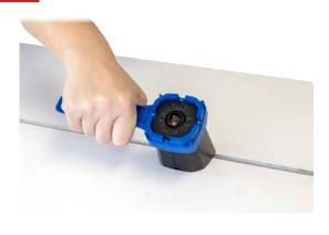
Place the VP-1477 removal tool over the pedestal with the indentation side facing up.
