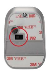
Turn the power switch to the ON position. Remove the 3M adhesive liner.
