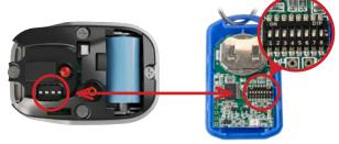
**IMPORTANT:** The code must match the 1-4 switches inside the IR Keyfob.
