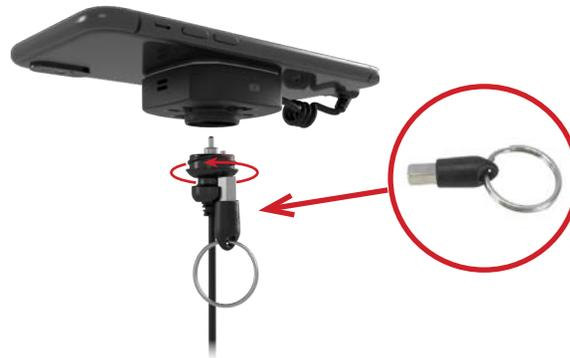
Use the magnet tool (VP-1446) to twist and release the boot from the sensor.
