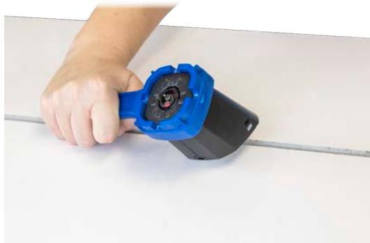
Gently twist the removal tool to break the adhesive bond.
