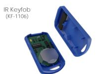
The EnCore and the Duo DIP switches need to match the keyfob.
