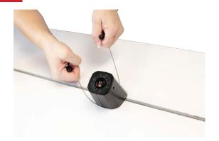
Optionally, you can use the V-44 removal tool. Wrap the removal tool's cable underneath the pedestal.
