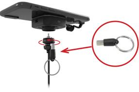
Use the magnet tool (VP-1446) to twist and release the boot from the sensor.
