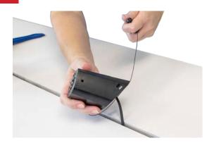
Alternate pulling the removal tool handles with each hand in a sawing motion until the pedestal is detached.
