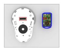
CR361: The IR Keyfob security codes are programmed to the CR361 the first time the system is armed. To change the security code, disarm the CR361, change the DIP switches, then rearm the system. The sensor and pedestal will be set to the new code.
