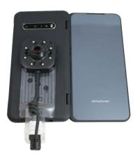
Remove the adhesive liner and adhere the sensor to the center of the case.
