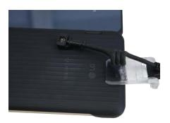
Remove the adhesive liner from the bracket. Attaxch the magnetic clip onto the charging port of the phone. Adhere the VP-1431C clip onto the case.
