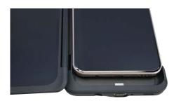
Remove adhesive liner from the AD-51. Place the device into the folding case and into the charging connector and snap into place.
