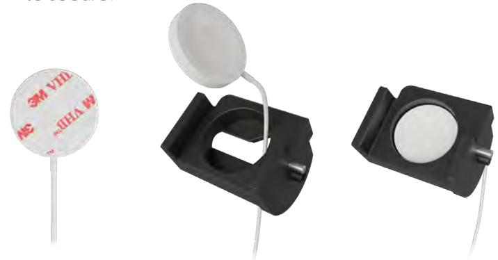
Apply the circular adhesive to the back of the watch puck. Thread the watch charging cable through the watch cradle for the specified device. Remove adhesive liner then adhere the charging puck inside the cradle.
