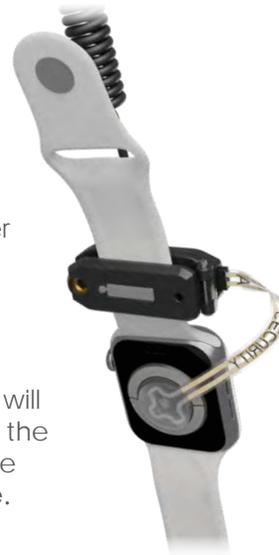
Remove adhesive liner and adhere the Flex Sensor to the back of the watch head.
