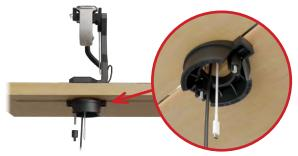
Screw the all-thread screws through the base of the stand. Then, thread the cables through the mounting ring and place the ring over the all-threads. Mount to the fixture with the two thumb nuts.
