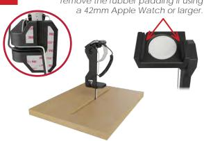
Rest the watch on the stand, and thread the sensor cable through the base of the stand. Route both cables through the fixture slot or through the back of the stand.
