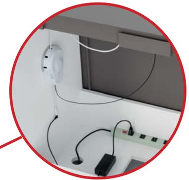
Ensure the tamper switch is depressed prior to securing the EnCore in place.
