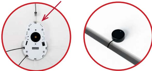
Adhere the IR dome close to the edge of the fixture slot. The IR Receiver will accept the keyfob's IR signal for the EnCore.
