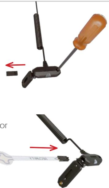
Insert the Flex Sensor (VP-1636) into the sensor.
