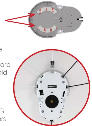
4 Plug the IR Receiver cable into the back port of the EnCore.
