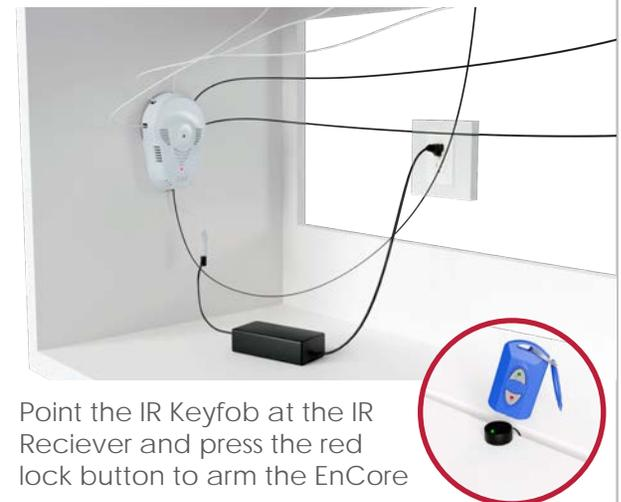
Point the IR Keyfob at the IR Receiver and press the red lock button to arm the EnCore
