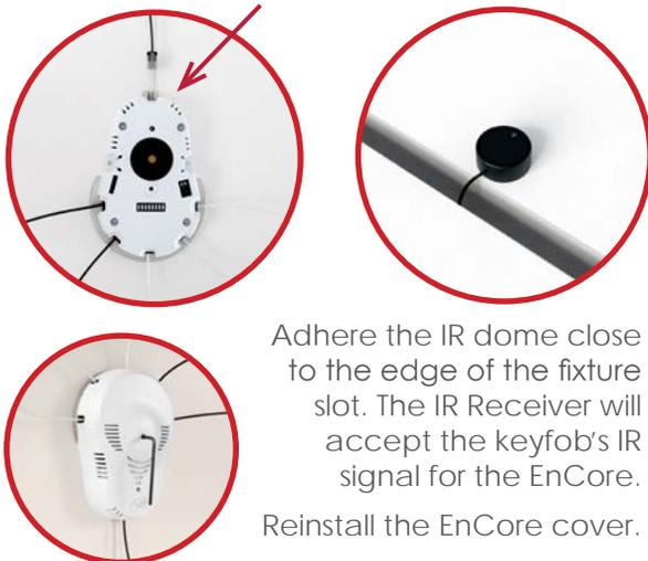
Adhere the IR dome close to the edge of the fixture slot. The IR Receiver will accept the keyfob's IR signal for the EnCore.
