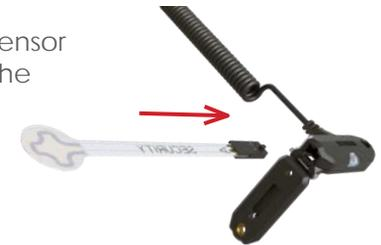
**8** Close the Slim Wearable Sensor onto the top watch band and tighten with the security driver.
