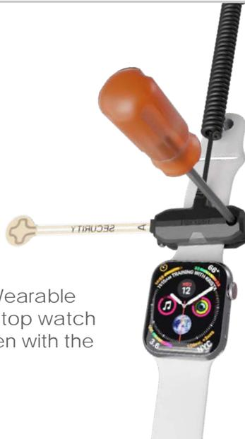
Close the Slim Wearable Sensor onto the top watch band and tighten with the security driver.
