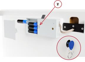
Close the battery compartment with the small flathead screw.
