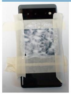
With a paper towel, dab the Novus to spread an even, thin layer onto the phone.
