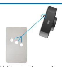
This is important because the tamper switch triggers the alarm; if the tamper switch does not get placed in one of those holes, it will remain pressed down, not going off if the phone is ever getting stolen.
